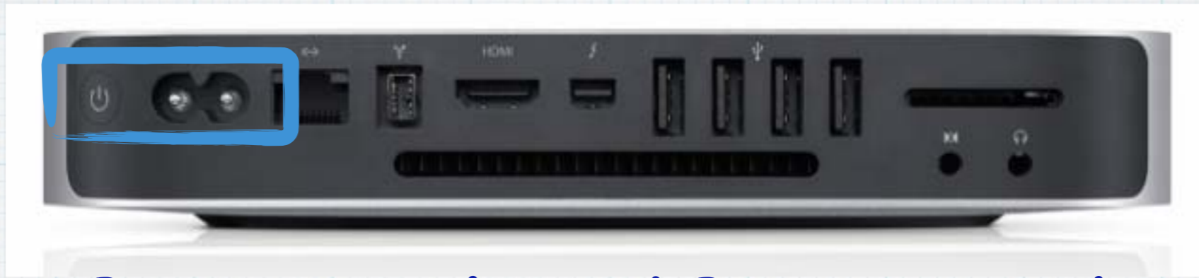
Power Supply and Power Switch
