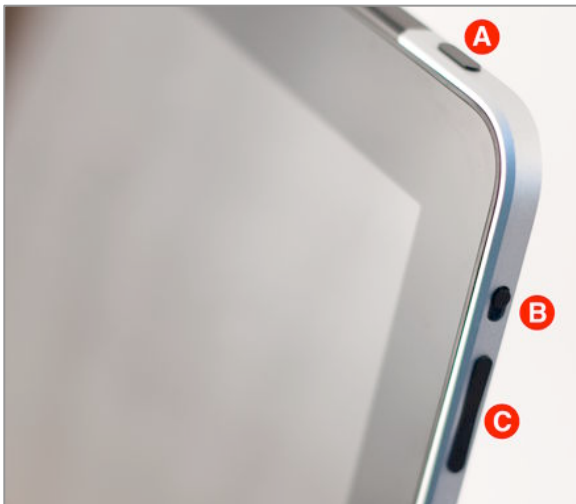
Figure 6: iPad in portrait position, upper right. (A) Sleep/Wake button, see Turn Your iPad Off and On . (B) Side switch (mutes background sounds and alarms, or locks screen rotation; see Rotate to Change Orientation ). (C) Volume up/down.
