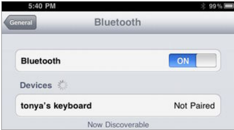
Figure 29: Discoverable devices appear in the Devices list. The very faint Bluetooth icon in the status bar by the battery indicator means that Bluetooth is on, but nothing is connected.
